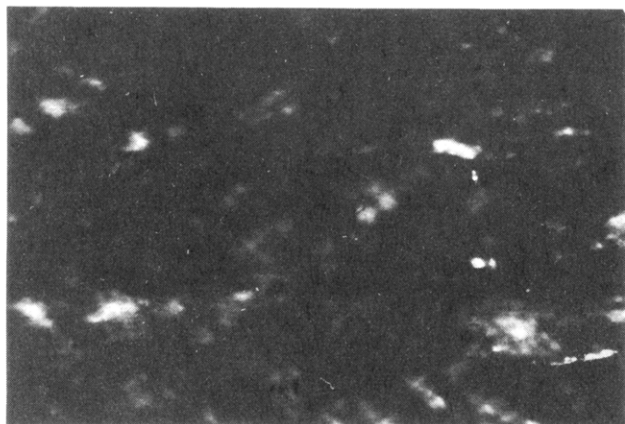
Figure 8. Optical micrograph between crossed polarizers of partially oriented film by shearing at 90 °C between fused quartz plates.
